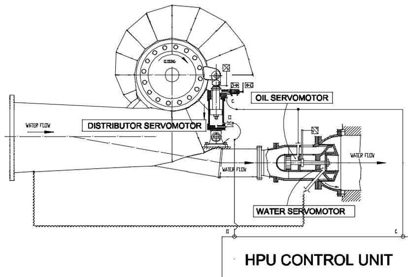
Fig. 2. Schematic drawing showing the power control of the PRV.
