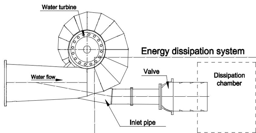
Fig. 1. Example of the EDS system attached to the horizontal Francis turbine with a horizontal Howel-Bunger type valve as PRV and an open space air outlet as the chamber.
