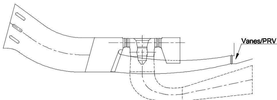
Fig. 4. Example of the EDS system with vaned PRV and submerged outlet to the tail race channel.
