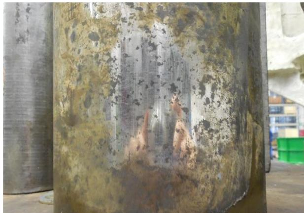
*Fig. 2. Pitting crevice corrosion on bearing counter surface*
