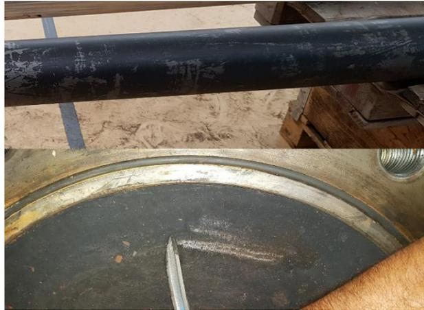
*Fig. 1. Galvanic corrosion; removal of material on the less noble material and deposits on more noble material*
