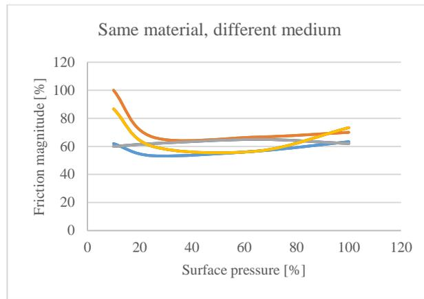
Fig. 3. Friction vs. surface pressure in different environments
