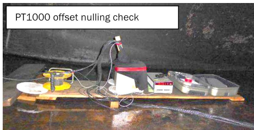
Figure 7 – Site offset check of Pt1000 temperature probes.
