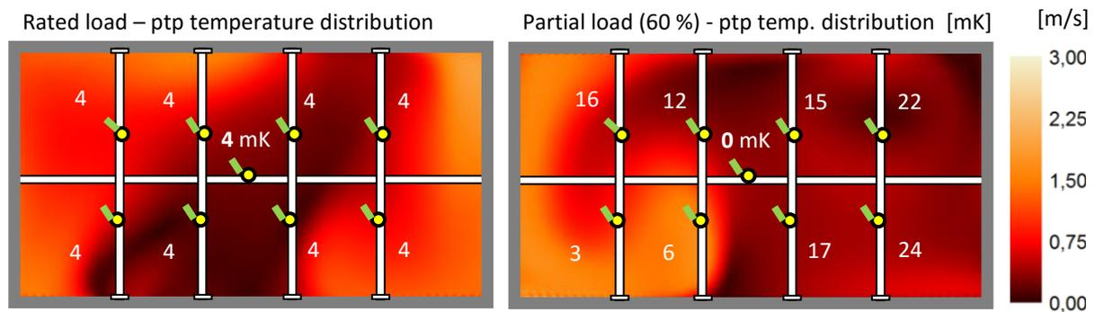
Figure 9 – Drat tube measured water temperature variations at location “20” compared to numerically calculated average velocities
