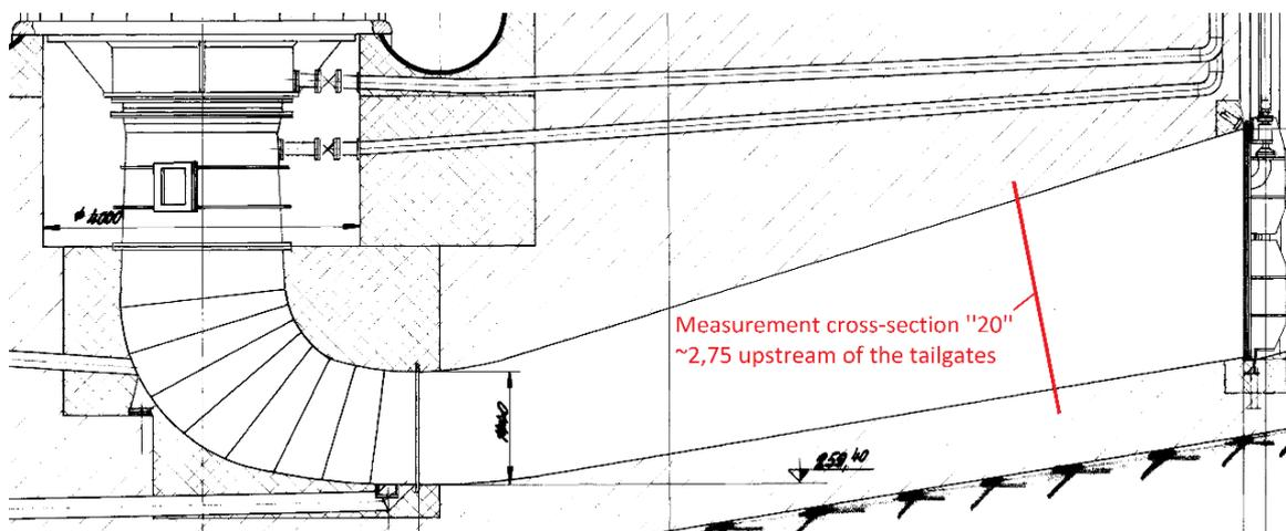
Figure 4 – Measurement cross-section downstream of the turbine.
