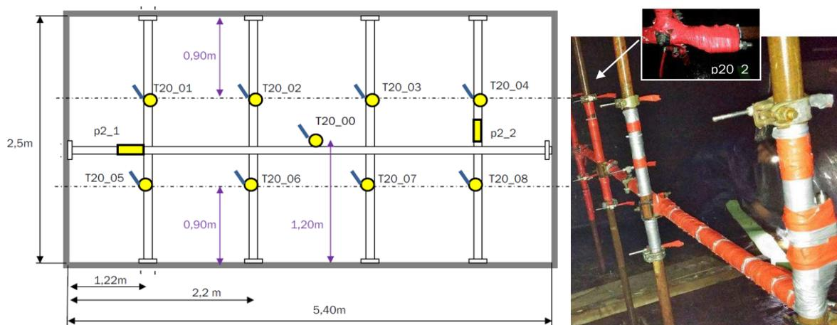
Figure 5 – Sensor layout at cross-section “20” downstream of the turbine.
